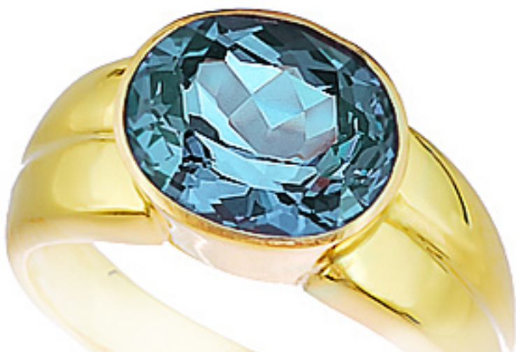
Fig. 18.: First synthetic color-change corundum was grown in 1909 and used as an alexandrite imitation. A lot of alexandrite heirloom jewelry contains synthetic corundum laced with vanadium to produce the color change.
