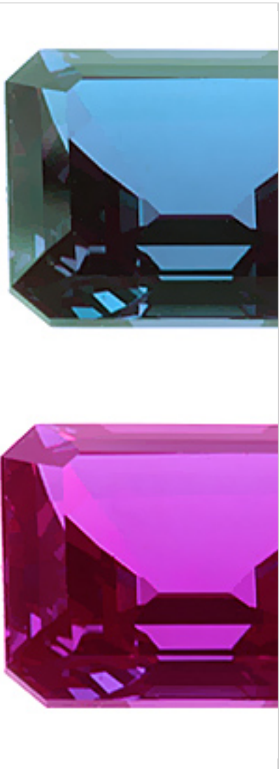
Fig. 20.: Czochralski or pulled alexandrite looks very clean, but contains curved striations visible with magnification and stone color is bluish under the daylight.
